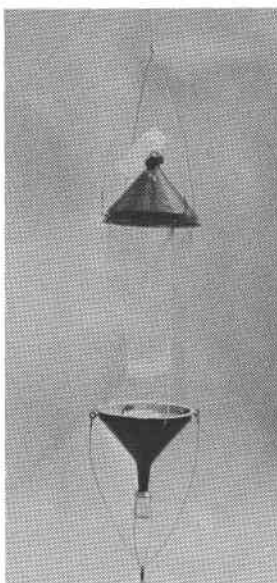
FIG. 1. Omnidirectional flight trap suspended by nylon cord. The funnels have been sprayed with brown and green paint and the collecting chambers have been filled with isopropanol. Note the upper collecting bottle seated snugly upon the foam rubber collar and held tightly in place by the elastic band.
